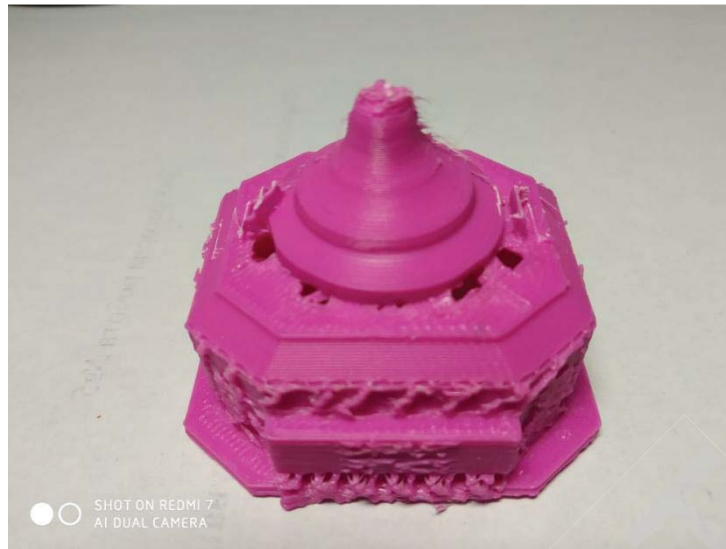
Fig. 6. - Illustration of offset layers in the middle of the printout
