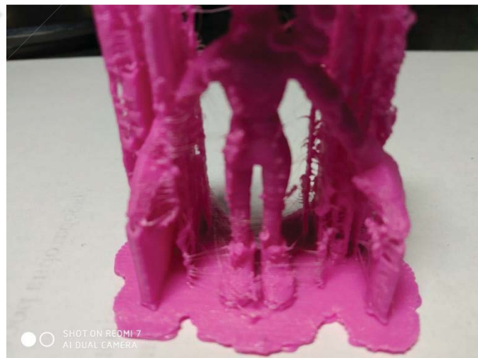
Fig. 9. - Illustration of the formation of "cobwebs" when printing
